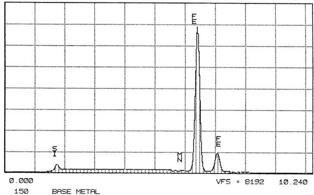
Fig. 27. Spectrum of elements representing base metal in Fig. 26.
