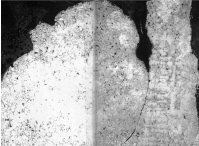
*Fig. 60. Photomicrograph showing quality of cast iron in vicinity of a filter segment where casting has sustained a cold shut and degenerate graphite; (50X, unetched condition).*
