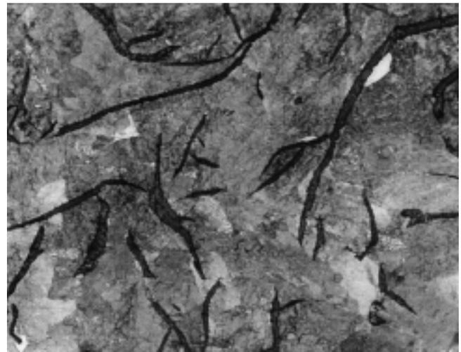
Fig. 59. Photomicrograph showing etched structure of casting, away from filter segment. Compare this structure with that shown in Fig. 56 near filter segment; (400X, nital etch).
