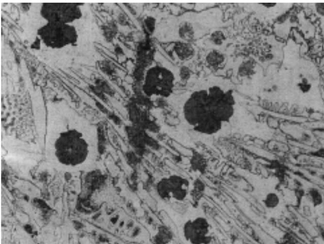
Fig. 9. Ductile iron photomicrograph illustrating primary carbides in a pearlitic ductile iron. Matrix is predominantly pearlite. The white angular constituents within pearlite are primary carbides; (400X, nital etch).
