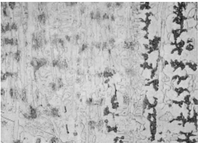
*Fig. 14. Photomicrograph showing primary carbides in gray cast iron with a predominantly ferrite matrix. Black constituent at right is graphite that appears to have precipitated after solidification; (100X, nital etch).*
