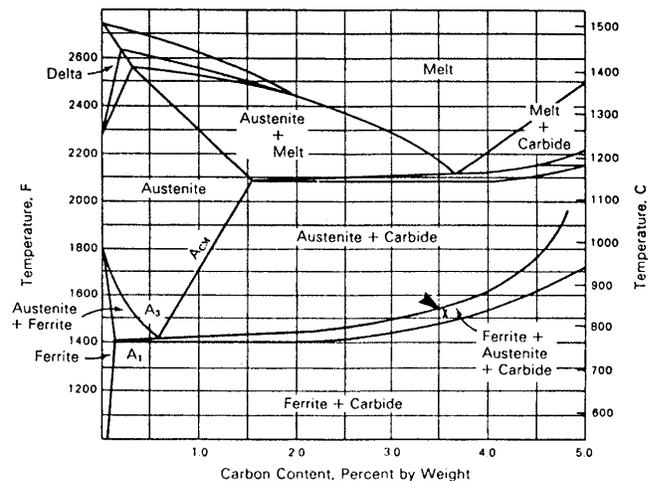
Fig. 37. Shown is iron-iron carbide-silicon ternary diagram sectioned at 2% silicon. "At the tip of the arrow head, X" shows austenitizing temperature reached, in three-phase region indicated by arrow, in two castings examined. Reprinted from "Iron Casting Handbook," American Cast Metals Association.
