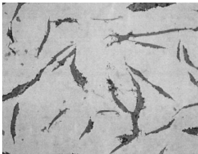
Fig. 30 Photomicrograph showing same area seen at lower magnification in Fig. 29. Note that graphite appears “fuzzy.” Also note that other graphite forms have precipitated within regions between flakes; (400X, unetched condition).
