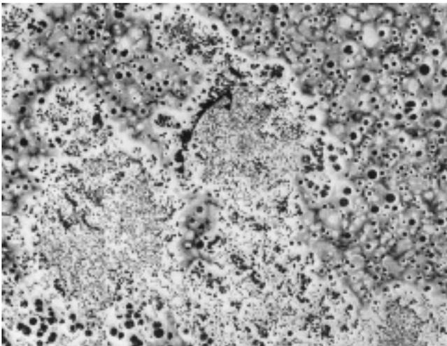
Fig. 25. Photomicrograph illustrating a dross defect in ductile iron. Dark constituent is pearlite; white constituent is ferrite. Note that ferrite concentrates with dross structure; (50X, nital etch).
