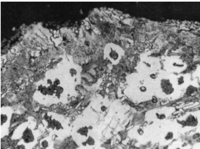
Fig. 5. Ductile iron microstructure illustrates poor graphite nodularity in matrix of pearlite (dark constituent) and ferrite (white regions surrounding graphite). Small, angular, white particles in matrix are primary carbides; (400X, nital etch).
