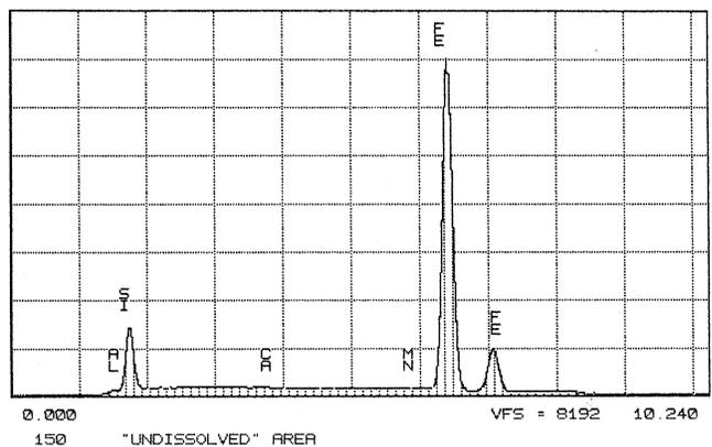
Fig. 28. Spectrum of elements representing partially dissolved inoculant in Fig. 26.
