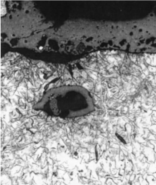
Fig. 56. Photomicrograph showing a cross section where a filter segment was trapped in microstructure; (50X, nital etch).
