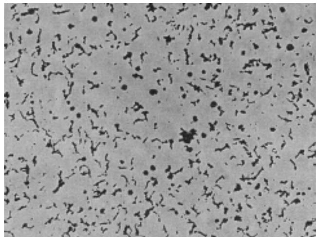
*Fig. 2. Photomicrograph of ductile iron shows unfavorable graphite nodule formation; (100X, unetched).*
