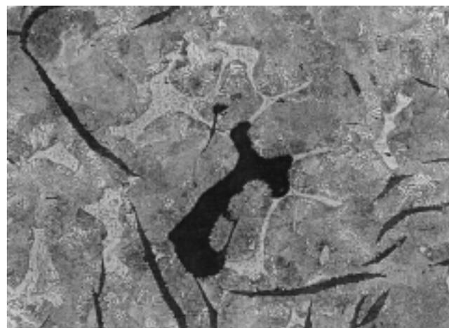
Fig. 22. Photomicrograph showing same void seen at lower magnification in Fig. 22. Note how void appears to be associated with steadite phase that is present in structure; (400X, nital etch).
