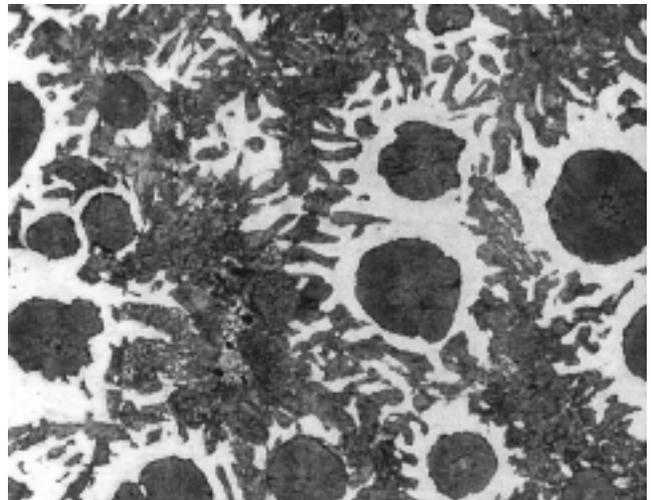
Fig. 36. Photomicrograph of same area shown at lower magnification in Fig. 35. This structure was intended to be annealed (100% ferrite); (400X, nital etch).
