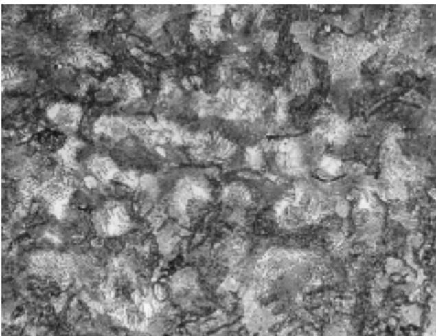
Fig. 53. Photomicrograph emphasizing coarse pearlite matrix in Fig. 51. See Fig. 55 for composition of matrix in this coarse area; (400X, nital etch).
