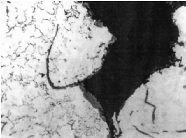
Fig. 48. Photomicrograph illustrating same area shown at lower magnification in Fig. 46. Note how graphite film at center left has been folded into metal. Also note that these individual "layers" have a graphite film liner; (400X, unetched condition).
