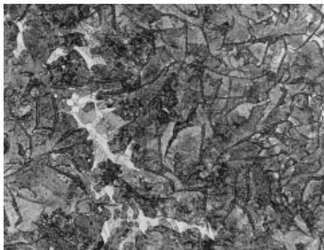
Fig. 18. Photomicrograph showing tertiary iron/carbon/phosphorus eutectic in a predominantly pearlite matrix gray cast iron; (400X, nital etch).
