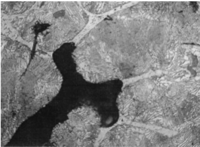
Fig. 23. Photograph showing same area seen at lower magnification in Figs. 21 and 22 to further illustrate how void that appeared as "shrinkage" in Fig. 20 is actually the absence of steadite; (1000X, nital etch).
