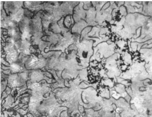
Fig. 52. Photomicrograph emphasizes fine pearlite in "hard spot" in Fig. 51. See Fig. 54 for composition of pearlite matrix in this "fine" area; (400X, nital etch).
