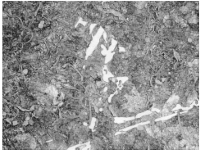
*Fig. 15. Photomicrograph showing primary carbides (white constituent) in a predominantly pearlitic gray iron matrix; (400X, nital etch).*
