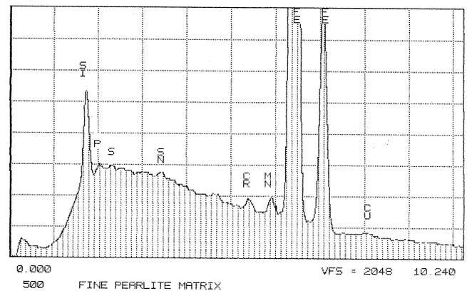
Fig. 54. Spectrum of elements representing fine pearlite in Fig. 52.
