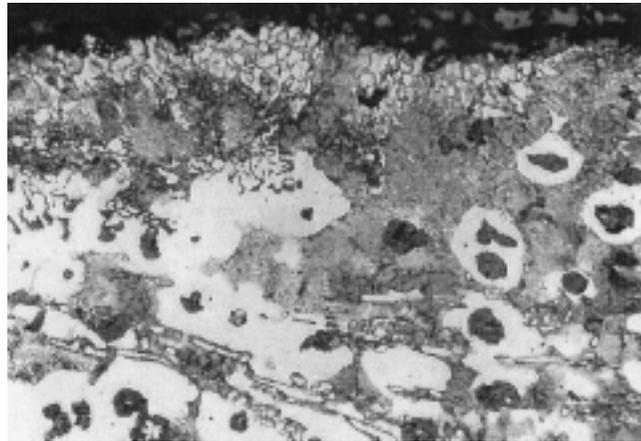
Fig. 4. Ductile iron microstructure shows flake surface graphite and nonspheroidal graphite. Dark matrix is pearlite; white is ferrite. Primary carbide is evidenced by blocky white structures occurring in pearlite and ferrite; (400X, nital etch).
