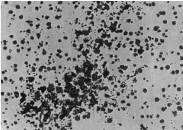
Fig. 24. Ductile iron microstructure with a dross type defect. This dross defect results from a reaction between magnesium dissolved in iron and oxygen in surrounding air; (100X, unetched condition).
