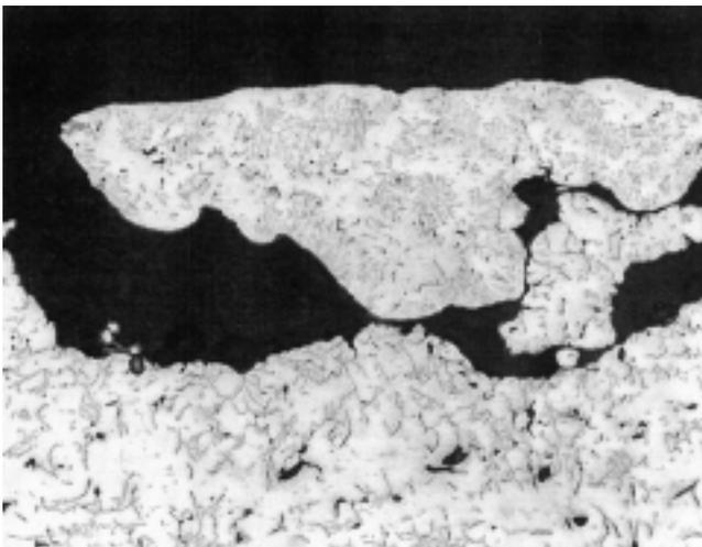
Fig. 47. Photomicrograph illustrating a cross section through one of the defective regions on casting. Note difference in graphite structure between three different "layers." These differences are characteristic of laps and cold shuts; (50X, unetched condition).
