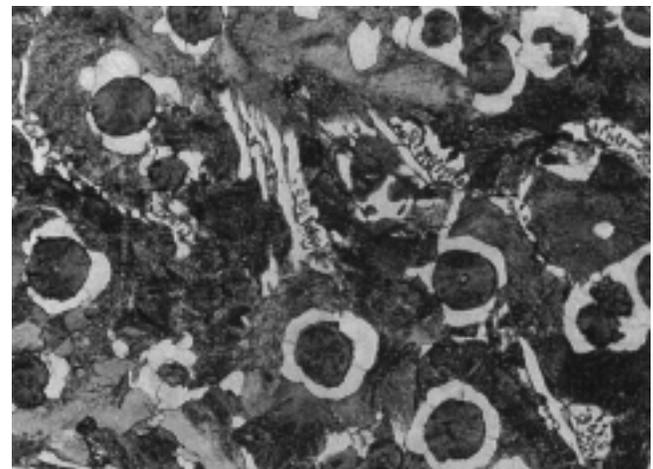
Fig. 11. Ductile iron photomicrograph illustrating primary carbides in a pearlitic ductile iron. Matrix is predominantly pearlite. The white angular constituents within pearlite are primary carbides; (400X, nital etch).
