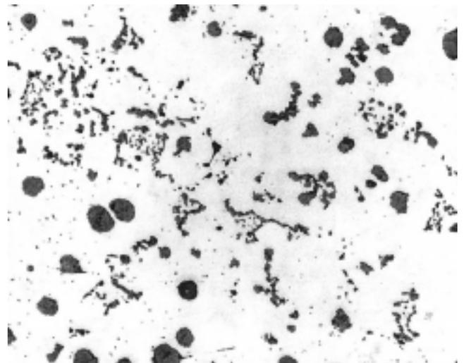
Fig. 46. At 100X, this photomicrograph shows microstructure's low graphite nodularity.
