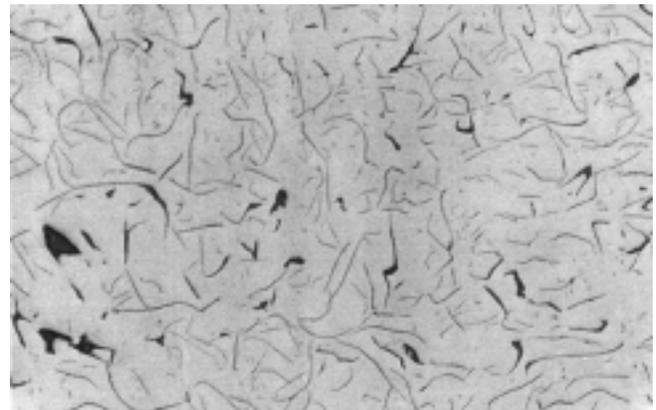
Fig. 58. Photomicrograph showing graphite structure of casting, away from defect; (100X, unetched condition).
