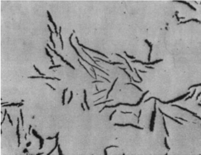
*Fig. 61. Photomicrograph illustrating "fat" graphite morphology associated with gray cast iron when nitrogen content becomes excessive (greater than 150 ppm); (100X, unetched condition).*
