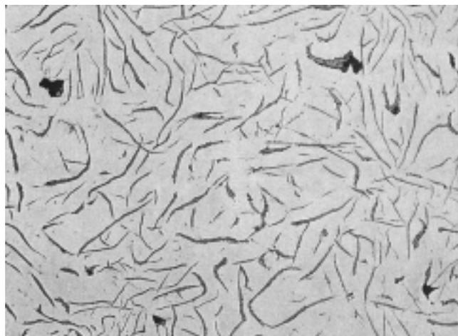
Fig. 29. Photomicrograph showing a “normal” graphite structure; (100X, unetched condition).
