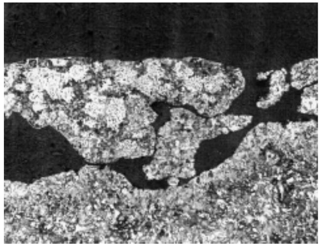
Fig. 49. Photomicrograph illustrating same area shown unetched in Fig. 46. This etched structure further exemplifies differences between individual layers; (50X, nital etch).
