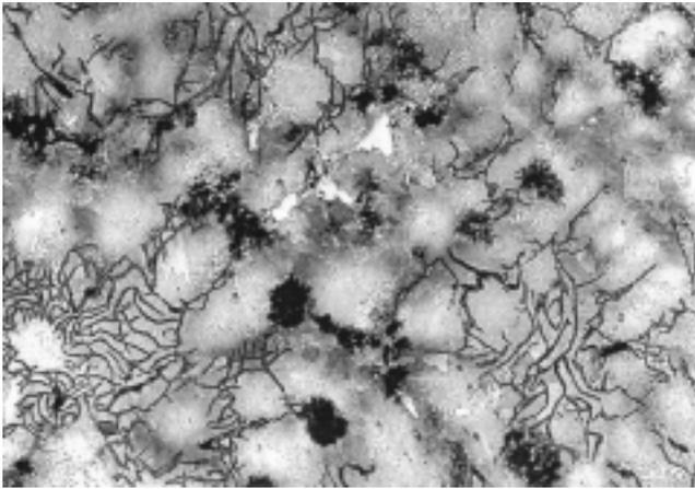
Fig. 32. Photomicrograph showing a pearlitic gray cast iron with Widmanstätten graphite. This area is shown at progressively higher magnifications in Figs. 33 and 34; (100X, nital etch).
