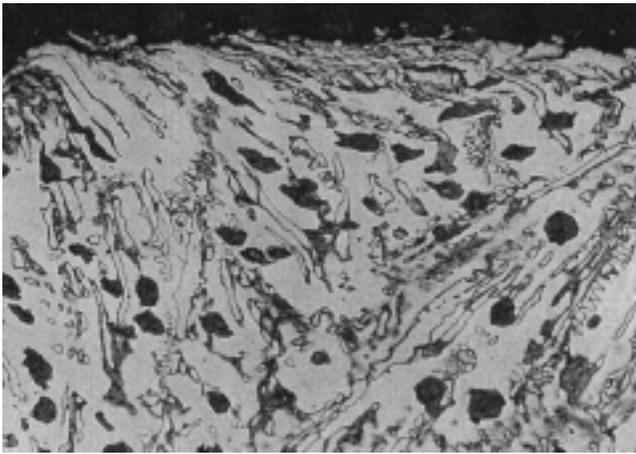
Fig. 3. Ductile iron microstructure is illustrated at a fracture site. Note pearlite (dark constituents) and ferrite (white constituents). White platelets are primary carbides resulting from inadequate inoculation or inoculant fade; (400X, nital etch).
