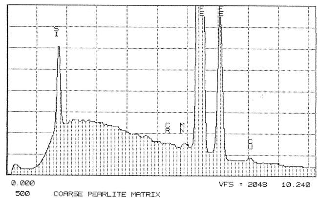
Fig. 55. Spectrum of elements representing coarse pearlite in Fig. 53.
