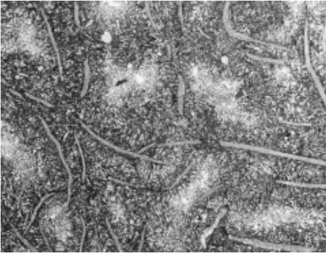
Fig. 40. Photomicrograph illustrating retained austenite in a martensitic gray cast iron. White angular constituent in structure is retained austenite; remainder of matrix is martensite; (400X, nital etch).
