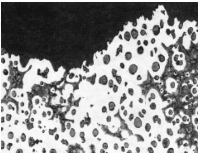
Fig. 44. At 100X, this casting is 70% ferrite (white area) and only 30% pearlite—20% below its specified pearlitic minimum.
