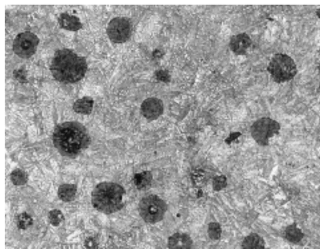
Fig. 39. Photomicrograph illustrating retained austenite in a martensitic ductile cast iron. Small angular white constituents (arrows) in matrix are retained austenite; matrix is martensite; (400X, nital etch).
