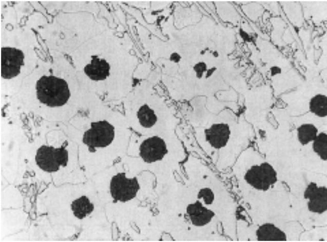
Fig. 7. Ductile iron photomicrograph with a ferritic matrix containing primary carbides. Predominant white matrix structure is ferrite; white angular constituents within ferrite are primary carbides; (400X, nital etch).
