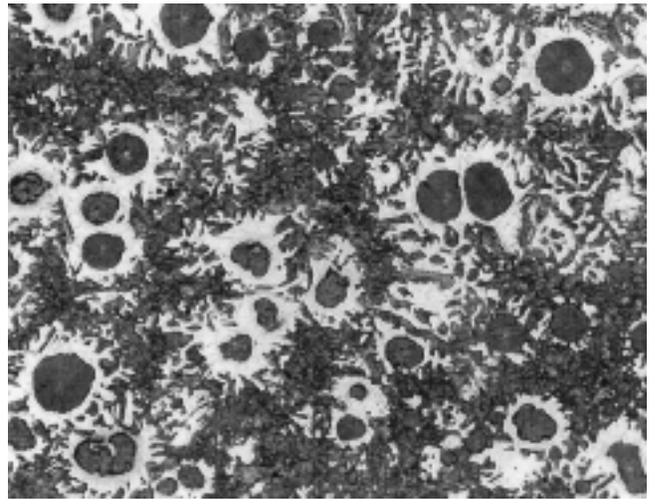
Fig. 35. Photomicrograph of ductile cast iron. This structure was intended to be normalized (100% pearlite); (200X, nital etch).
