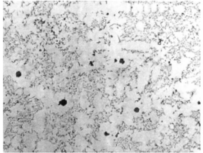
*Fig. 62. Photomicrograph showing spheroidal graphite in a gray iron casting; (400X, unetched condition)*
