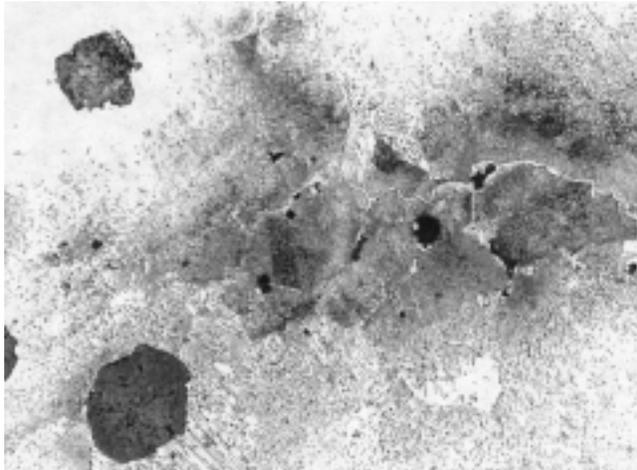
Fig. 42. Photomicrograph showing high incidence of intercellular carbides in casting. See Fig. 43 for composition of carbides; (400X, nital etch).
