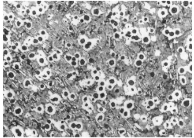
Fig. 10. Ductile iron photomicrograph illustrating primary carbides in a pearlitic ductile iron. Matrix is predominantly pearlite. The white angular constituents within pearlite are primary carbides; (200X, nital etch).
