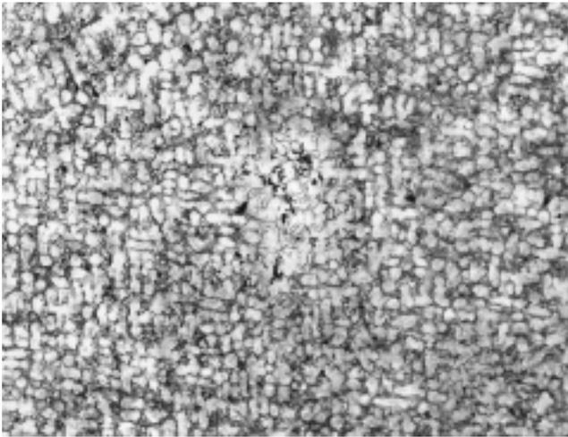
Fig. 51. Photomicrograph showing "hard spot;" (50X, nital etch).
