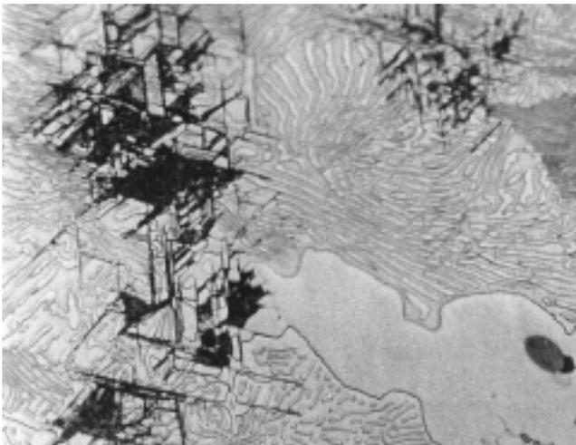
Fig. 34. Photomicrograph showing same area seen at lower magnification in Figs. 32 and 33 to further illustrate graphite precipitated on crystallographic planes; (1000X, nital etch).
