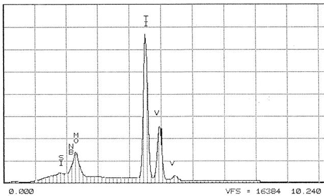
Fig. 43. Spectrum of elements representing intercellular carbides in Fig. 42.
