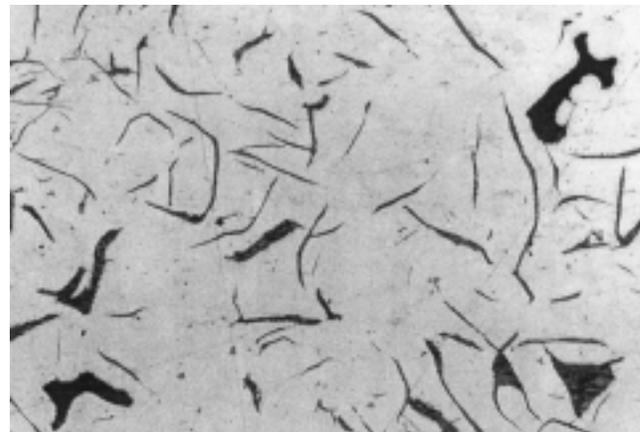
Fig. 20. Photomicrograph showing presence of a "shrinkage" void in a thin section at upper right; (200X, unetched condition).
