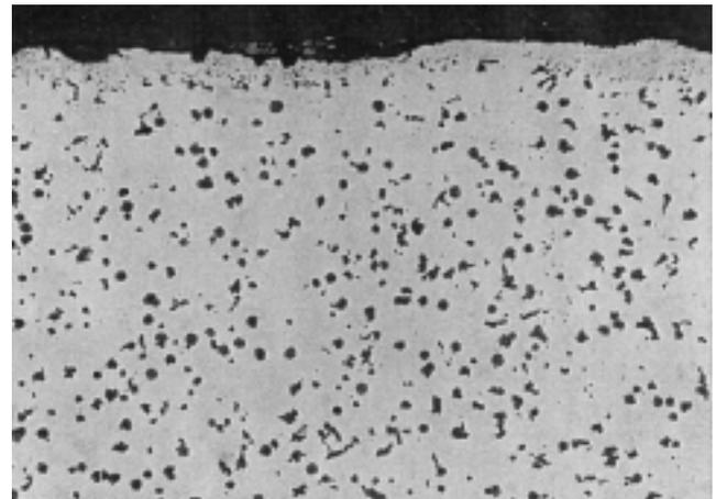
*Fig. 1. Poor ductile iron nodularity caused this utility cover plate to fail; (100X, unetched).*
