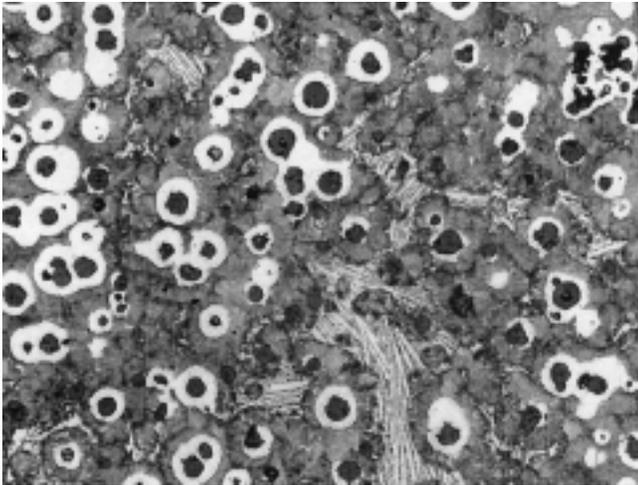
*Fig. 13. Ductile iron microstructure illustrating inverse chill primary carbides in a pearlitic ductile iron. Needle-like carbides toward middle bottom of photograph are inverse chill; (200X, nital etch).*
