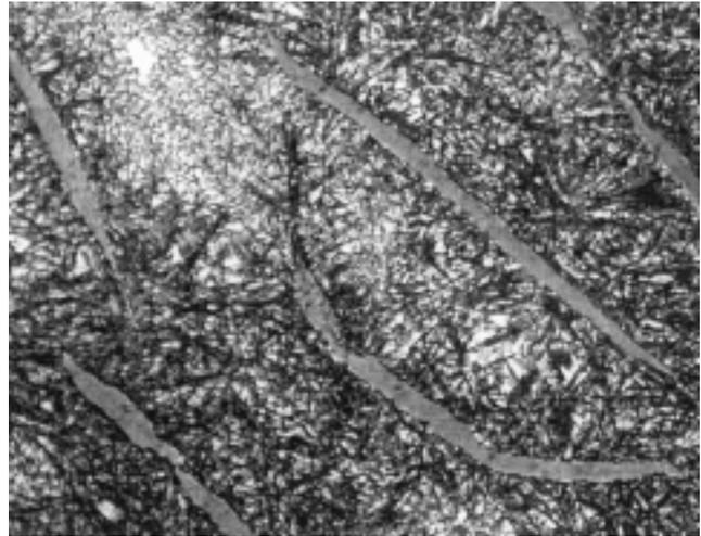
Fig. 41. Photomicrograph illustrating retained austenite in a martensitic gray cast iron. White angular constituent is retained austenite; remainder of matrix is martensite; (1000X, nital etch).
