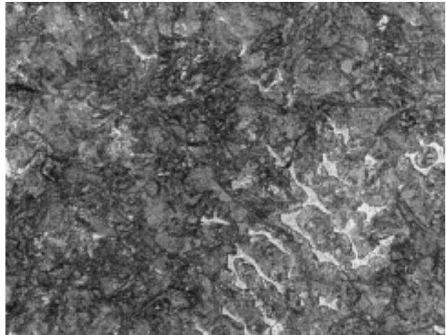
*Fig. 16. Photomicrograph showing steadite in a predominantly pearlitic gray cast iron; (200X, nital etch).*
