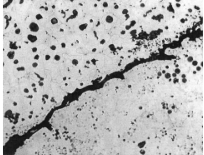
Fig. 26. Photomicrograph illustrating a line of demarcation between a "normal" structure and a partially dissolved inoculant area (200X, unetched condition) (see Figs. 27 and 28).
