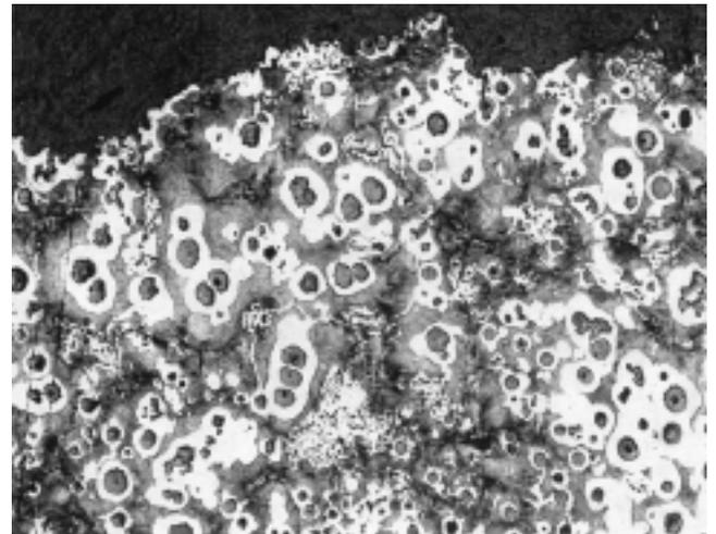
Fig. 45. At 100X, casting's pearlitic content is acceptable (80%).
