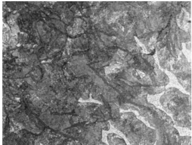
*Fig. 17. Photomicrograph showing same area seen at lower magnification in Fig. 16 to illustrate "pepper marks" within steadite plate constituent; (400X, nital etch).*
