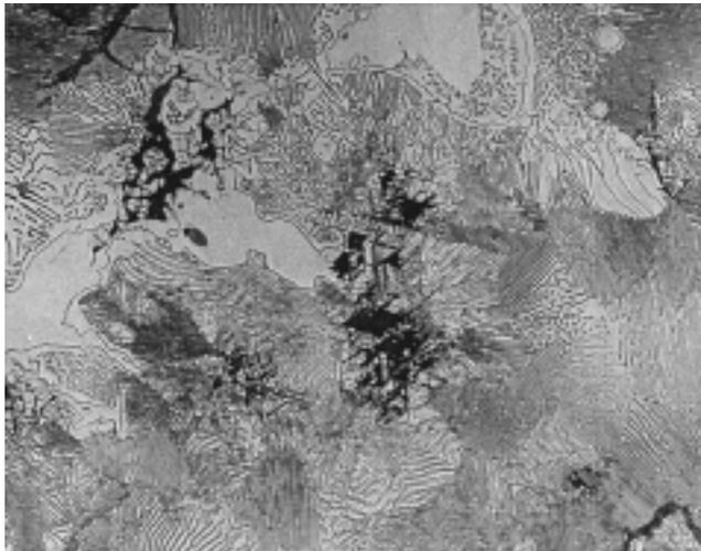
Fig. 33. Photomicrograph showing same area seen at lower magnification in Fig. 32 to illustrate Widmanstätten form of graphite. Note that graphite has precipitated at angles representative of crystallographic planes; (400X, nital etch).
