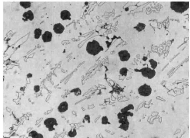
Fig. 6. Ductile iron photomicrograph with a ferritic matrix containing primary carbides. Predominant white matrix structure is ferrite; white angular constituents with ferrite are primary carbides; (400X, nital etch).
