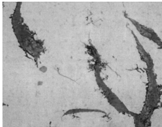
Fig. 31. Photomicrograph showing same area seen at lower magnification in Figs. 29 and 30. Note that “fuzzy” graphite is consequence of small fingers of graphite growing on sides of graphite flakes. Also note graphite forms with thin graphite forms in between graphite flakes toward middle and middle top; (1000X, unetched condition).
