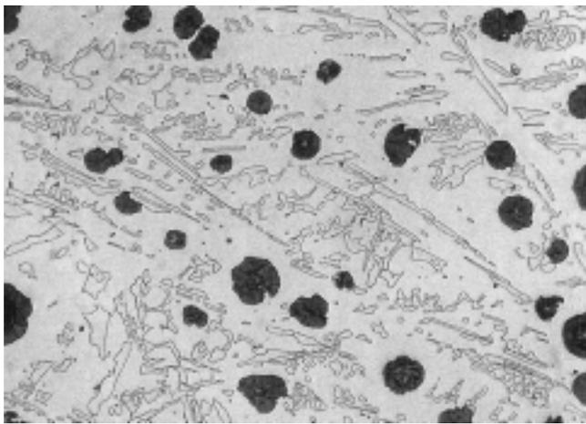
Fig. 8. Ductile iron photomicrograph with a ferritic matrix containing primary carbides. Predominant white matrix structure is ferrite; white angular constituents within ferrite are primary carbides; (400X, nital etch).
