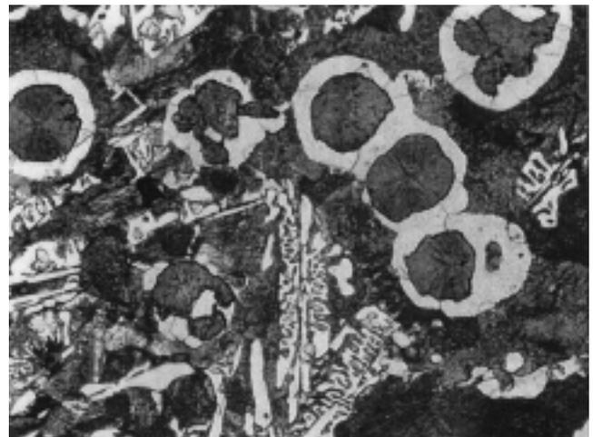
Fig. 12. Ductile iron microstructure illustrating primary carbides in a pearlitic ductile iron. Matrix is predominantly pearlite. The white angular constituents within pearlite are primary carbides; (400X, nital etch).
