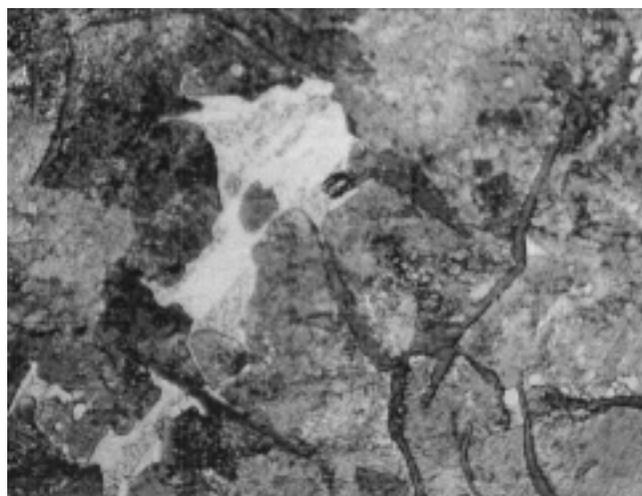
Fig. 19. Photomicrograph showing tertiary iron/carbon/phosphorus eutectic in a pearlite matrix gray cast iron; (1000X, nital etch).
