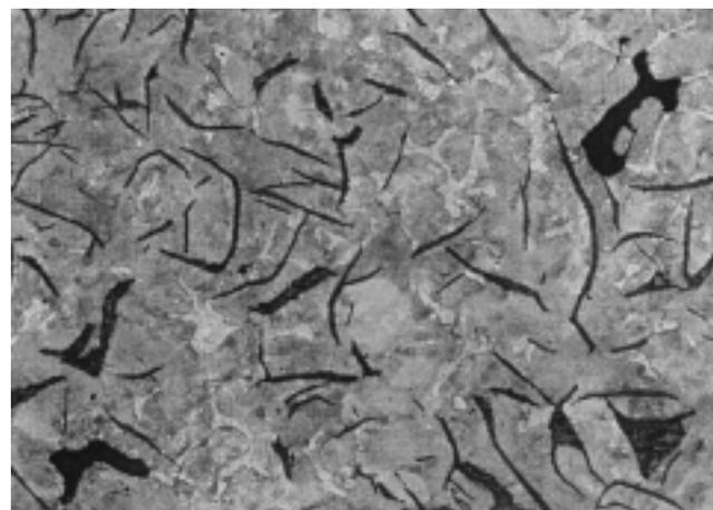
Fig. 21. Photomicrograph showing same area seen unetched in Fig. 20 to further illustrate nature of matrix associated with void. Matrix is predominantly pearlite; white constituent is steadite; (200X, nital etch).
