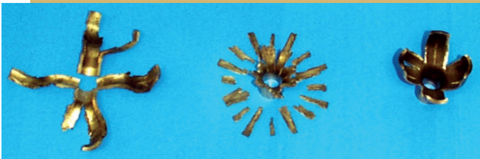
Gas-gun cylinder experiments provide a direct way to quantify differences in material failure. Even under identical drives, differences in cracking and failure are obvious.
