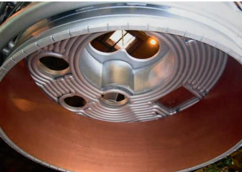
LF roof on the Siemens Metals Technologies workshop ready for delivery
