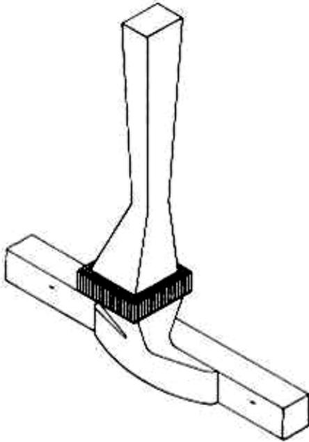
Fig.36 Filter in the gating system of a mould with vertical parting plane
