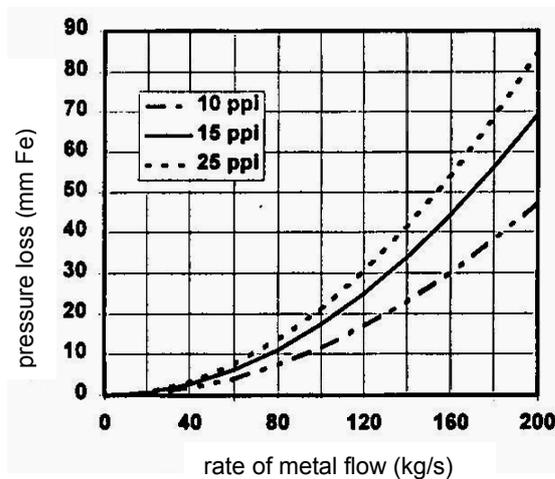
Fig. 31: Pressure loss caused by a filter
