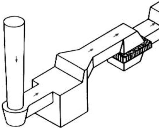
Fig. 41: Filter installation for in-mould modification
