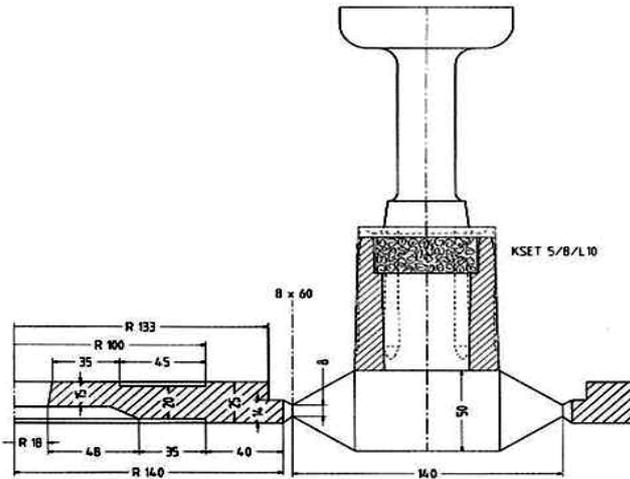
Fig. 34: Closed riser extension with filter
