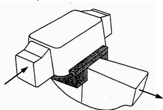
Fig. 32: Recommended method of filter positioning for steel casting
