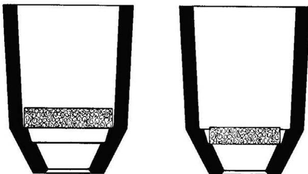
Fig. 33: Pouring cups with filters
