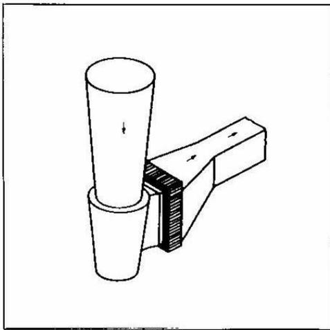
a) Vertical position of filter close to the sprue
