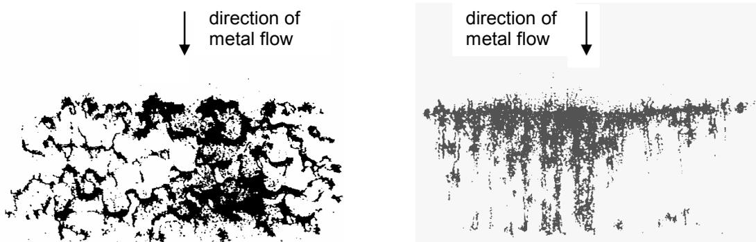
Fig.22: Sulphide inclusions captured in a foam filter and in a pressed filter with straight channels
