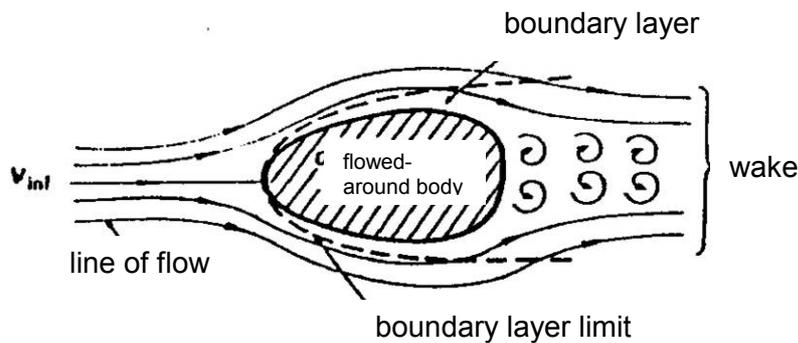
Fig. 42: Appearance of wake when metal is flowing through the filter
