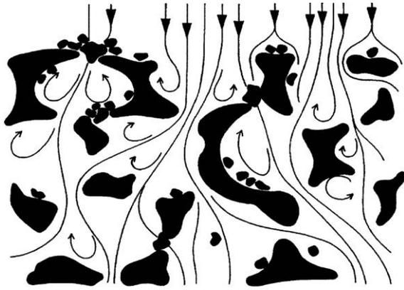
Fig. 20: Flowing in a foam filter
