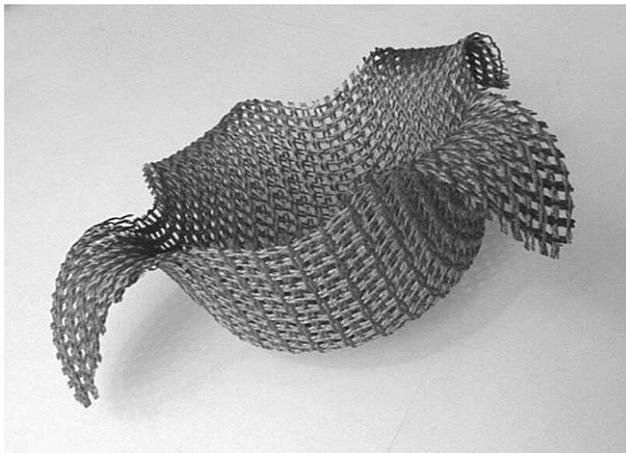
Fig.14: Cloth filter for the pouring basin
