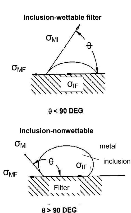
Fig. 8: Filter wetted by liquid inclusion
