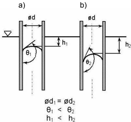
Fig. 24: Resistance to filter priming:
