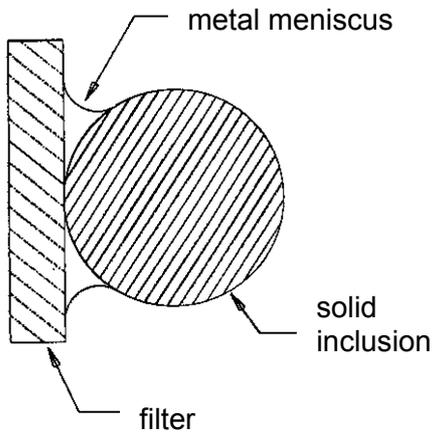
Fig. 9: Solid inclusion captured on filter wall
