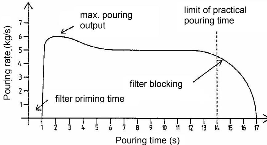
Fig. 23: Curve of filter flow rate
