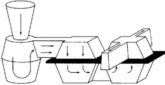
Fig. 13: Positioning filters in a mould
