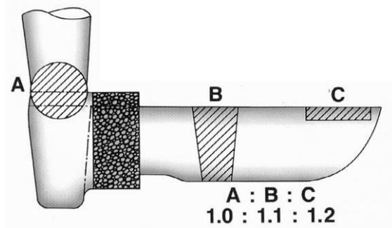
Fig. 28: Example of the gating system design with vertically placed filter
