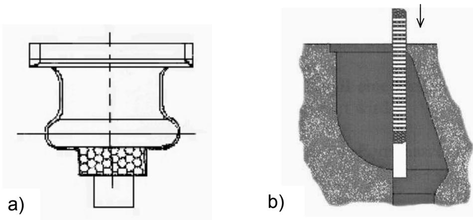
Fig. 35a,b: Filter insertion in the pouring basin of moulds with vertical parting plane
