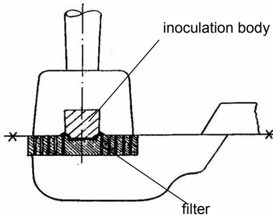
Fig. 39: Inoculation bodies on a filter
