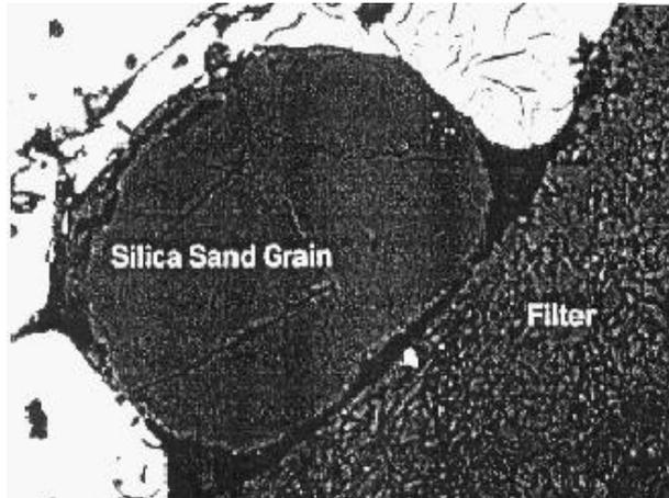
Fig. 3 Solid inclusion fixed to a filter wall
