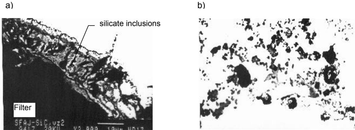
Fig. 2 Examples of inclusions in ductile iron
