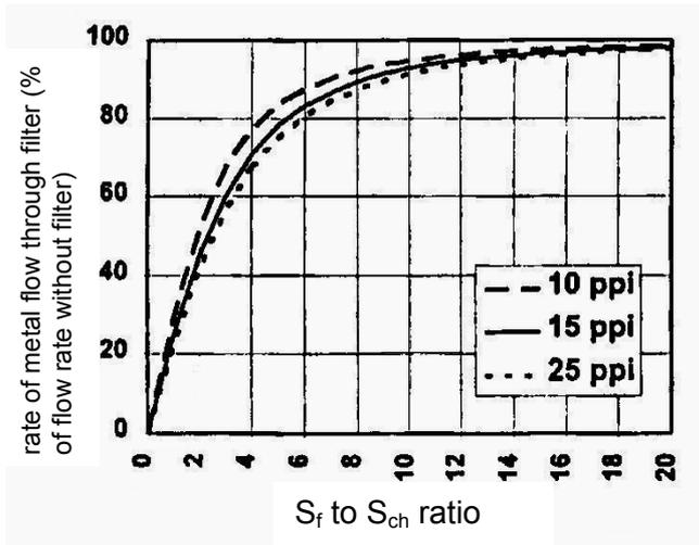
Fig. 29: The effect of filter size on pouring time extension
