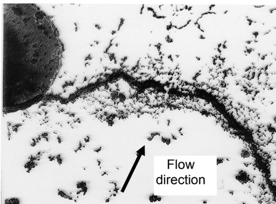
Fig. 21: Inclusions forming a bridge in foam filter
