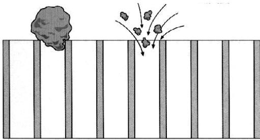
Fig. 5: Filtration by straining
