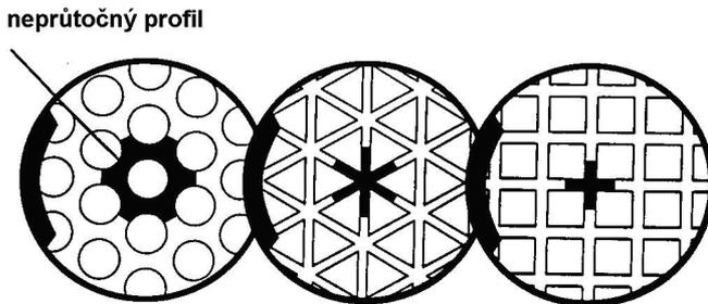
characteristic of filters. The area formed by ceramics constrains the filter cross section - see Fig. 11. Unless the metal flow is to be reduced by passing through the filter, it is necessary to increase the filter cross section in comparison with the runner cross section so that the total cross section of all holes is identical to that of the choke in the gating system. The proportion of the flow cross section in the total area amounts to some 15 – 80%,
