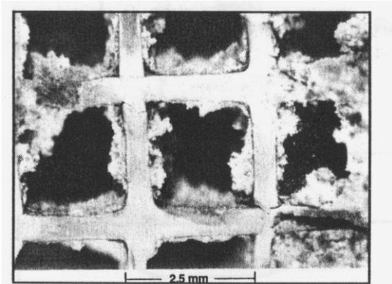
Fig. 17: Extruded filter with captured inclusions
