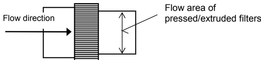
Fig. 30: Filter flow area
