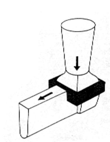
Fig. 26: Direct pouring on a filter
