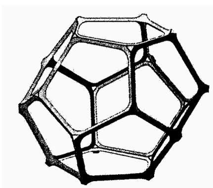
Fig. 18: Foam filter cell
