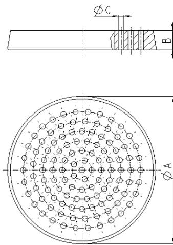
Fig. 10: Ceramic strainer cores
