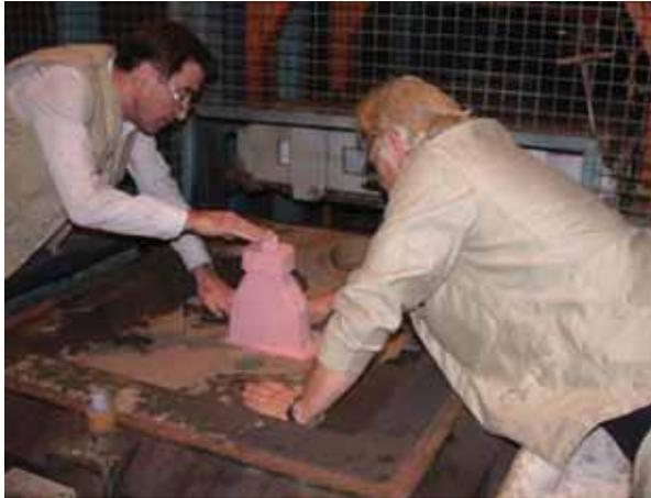
**Figure 4** Moulding of inner wheel arch
