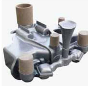
Figure 11 Outer wheel arch raw casting
