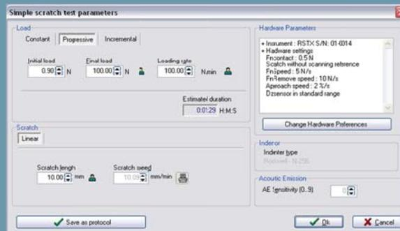
2. Export the test protocol via USB stick to the Revetest Xpress
