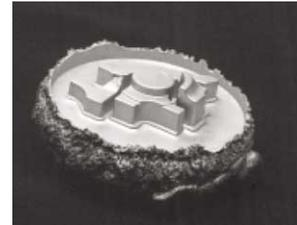
As-deposited H13 tool steel die for die casting applications.
