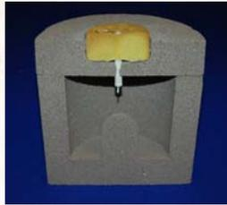
Test cup for investigation of metal expansion penetration mechanism
