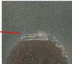
Cross section of a penetration test cup
