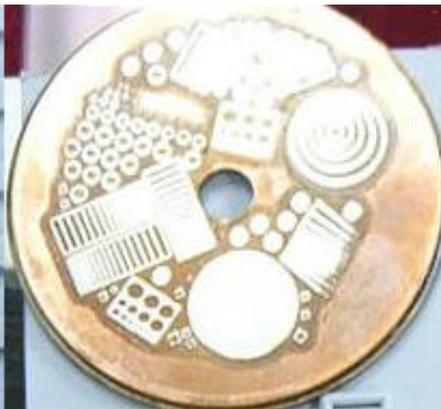
Nickel features electroplated on tool steel base
