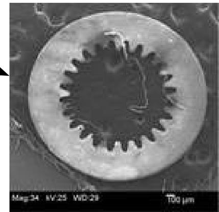
micrograph of MW sintered gear
