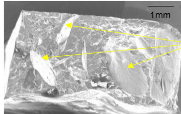
Alumina fracture surface
