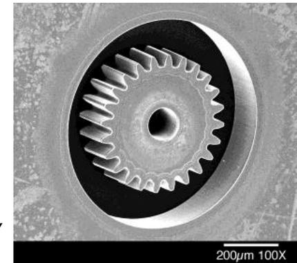
micrograph of gear mold
