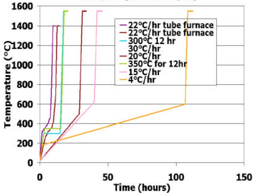
Microwave debinding and bisque of alumina combustor MOR bars
